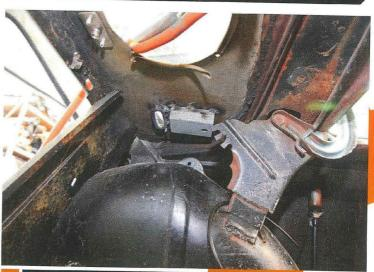
As with the position of the top hat, the position of the guide ring is also critical. Charisma got the positioning of both spot-on — the belt doesn't touch anything except the vinyl on the parcel shelf. A squirt of pressure-pack black was applied to stop the dreaded rust emerging; yes, I noticed the beginnings of corrosion in some of the surrounding areas, which will need attention in the not-too-distant future.
