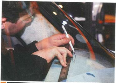
As with any modification, measure everything several times if you want it all to work properly. When determining where to position the mechanism, you need to verify there is enough room to mount the reel while ensuring the belt emerges at a point where it will sit comfortably on the passenger's shoulder and minimise the risk of it slipping off in an accident, so don't mount it too far inwards or outwards.
