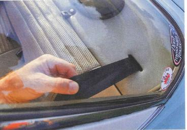
Once everything is bolted correctly back into place, check that all the belts move freely without rubbing, snagging or binding. Check that the ELR mechanism works by giving it a swift tug and then test to see that it also fully retracts. This will ensure a long service life and avoid the embarrassing situation of driving down the road with the tinkling sound of an unspooled seatbelt dragging along behind.
