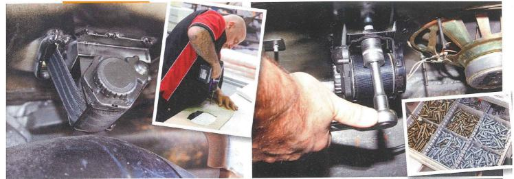
So that the buckle doesn't have to be threaded up through the parcel tray, the belt's fed in from the top and wound onto the reel. This means the parcel tray cover needs to be fitted before bolting the reels in place. After marking the cover from underneath, a slot was carefully cut into it. Enough vinyl was left around the slot so it could wrap through the hole and be stapled underneath for a neat, professional finish.
