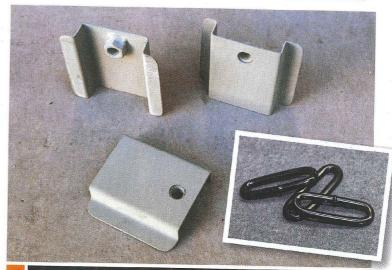
Charisma fabricated these top-hat mounts to which the reels will be bolted. The stepped design accommodates the captive nut and gives the webbing a better angle to run through the slot in the parcel shelf. It's critical the belt doesn't rub on any sharp edges as frayed belts are dangerous and a roadworthy failure in the making. Welding in guide rings gives the belts a smooth, solid surface to run over.
