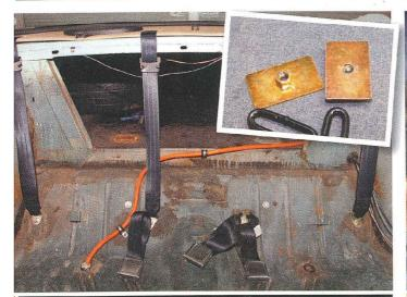
If your car has OEM seatbelt mounts (my Rambler does) then simply bolt up the buckles and ends. If not, you'll need to use 75x50mm reinforcing plates. The large size is to prevent them pulling through the floor in an accident — 3mm-thick plates are preferable to 6mm as they'll deform rather than tearing through the metal. These plates must sit flush against the metal and some massaging may be required.
