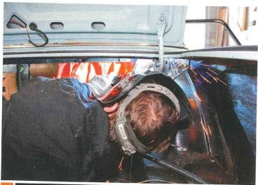
I could have done all the fabrication at home myself but instead I had Charisma Custom do the dirty work. To cut the slots in the metal parcel tray, a half-inch hole was drilled at either end (using a right-angle attachment on the drill), then a nibbler was used to remove the remaining material. Welding the top hats and guide rings while hanging upside-down in the boot was both uncomfortable and challenging.
