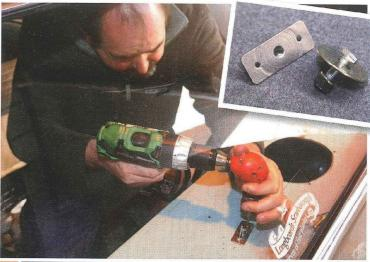
This child anchorage (inset, left) is the same design used by Mercedes Benz. They're better and simpler than the nut, bolt and large washer (inset, right) supplied with the harnesses. As with the seatbelt reinforcing plates, child anchorages can be welded or riveted as the only requirement is that they remain in place when the bolt is removed. After drilling the holes from the top, they were riveted in underneath.
