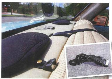
In the foreground you can see the tab that bolts to the top side of the anchorage point. Attached to the belt is a clip with a safety spring (inset) that can't be removed unless you hold your head and tongue at just the right angle. The trick is to lift the buckle vertically and then press the retaining spring. Careful thought must go into correctly locating the tab so as to have enough room to perform this awkward task.
