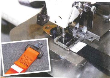
The buckles and end-mount tabs are affixed to the webbing via stitching that can only be done by a certified machine and machine operator. The fully automated machine does the specialised routine in only seven seconds. In a tensile strength test, the webbing broke before the stitching let go! The all-important white tag (inset) shows the belt meets the relevant Australian and NZ standards, plus date of manufacture.
