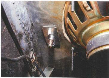
The ideal anchorage point is right where the 6x9s are positioned. However, the speakers were there long before the kids came along. If the anchorage points were installed behind the 6x9s, the close proximity of the rear screen would make it very difficult to attach and remove the tether straps. Instead, Charisma placed the anchors in front, using 5/16 UNC bolts to secure the top mounting tabs (see next step).
