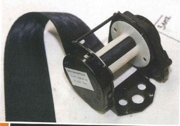
These are the retractable inertia reel assemblies that will be installed under the Rambler's parcel tray. They are a universal-fit Emergency Locking Retractable (ELR) design that's available in three different mounting configurations: vertical, topmount and underhung. The units look very similar but there are slight differences in their locking mechanisms to suit the different mounting orientations.
