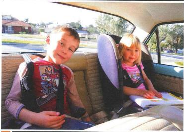
The Rambler's rear lap belts required the use of difficult-to-adjust and untidy H-harnesses for the kids. I was never happy with them as the kids couldn't buckle themselves in and they never fitted correctly. While the new retractable lap/sash belts solved this problem, it didn't address the fact that we were about to add twin baby girls to the brood. Time to sort the child restraint situation once and for all.
